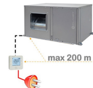
Electrical connection for distances exceeding 10m
